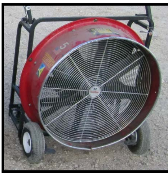
Honda PPV fan (not functional)
